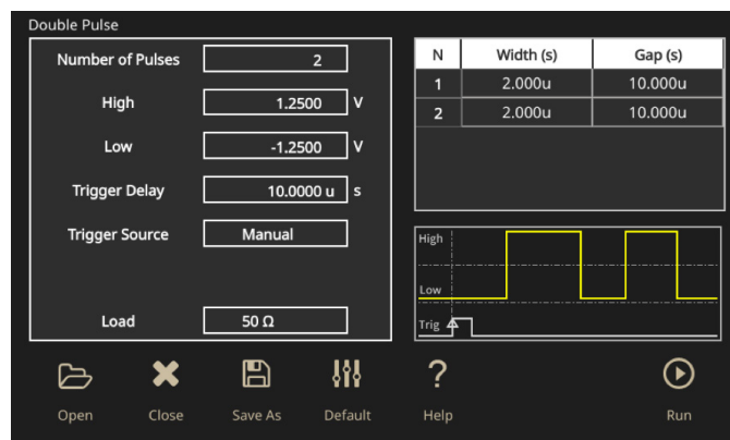
Figure 17: Double Pulse Test Application on the AFG31000 enables easy configuration of multiple pulses with different widths.
